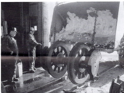
Ed Beard (l) and Steve Montano direct the moving of a driver set from engine 487 to the wheel lathe in the Chama enginehouse. (All photos January 2003.)
