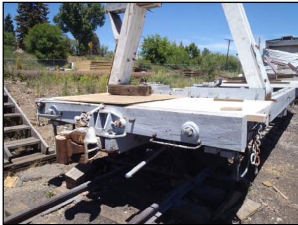
“A” end coupler installed.
