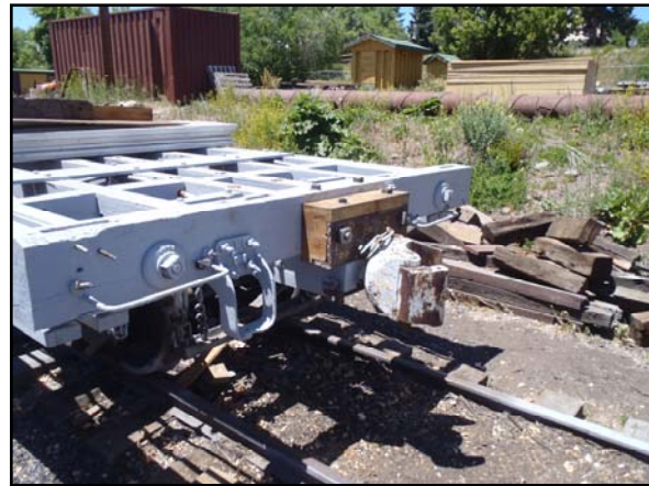
”B” end coupler installed.
