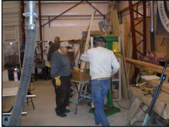
Spero Bettalico gets instructions from Team Leader Russ Hanscom on the drilling of the Plates needed either 2 or 4 holes drilled. Over 500 holes in all.
