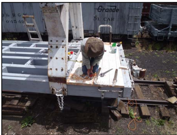
Team Leader Russ Hanscom drilling holes for the outer supports/hold-downs for the horizontal outriggers.
