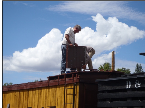
Making adjustments to ice hatch.
