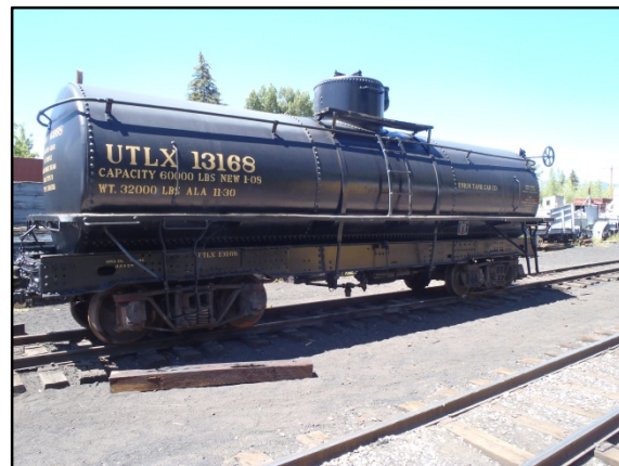
UTLX 13168 with newly installed arch-bar trucks under both ends of the car.
