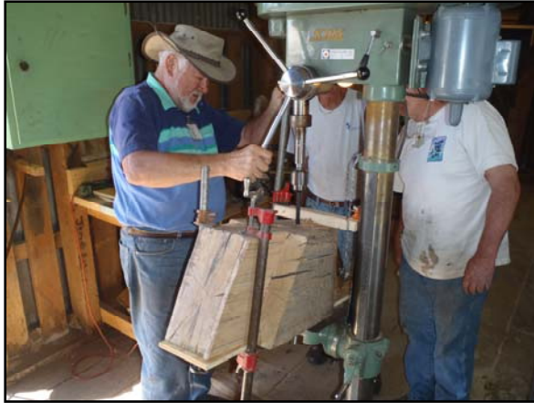
Herb Knoesel is drilling two angled holes in the crown block for 1 1/4 " vertical tie rods. The crown block forms the core of the top of the A frame assembly.
