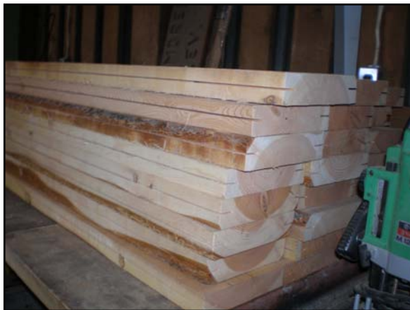
First cuts to make the ship lap pattern have been made.
