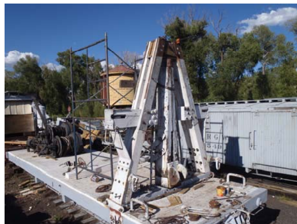
The double drum winch assembly has been moved back onto the car and the pivot post has been secured.
