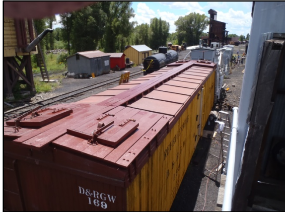
Hatches and catwalks newly hand painted.
