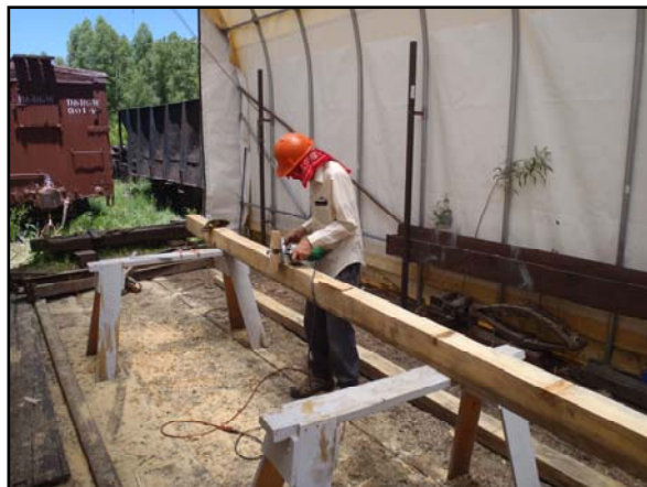
George Detwiler working on an upper side sill.
