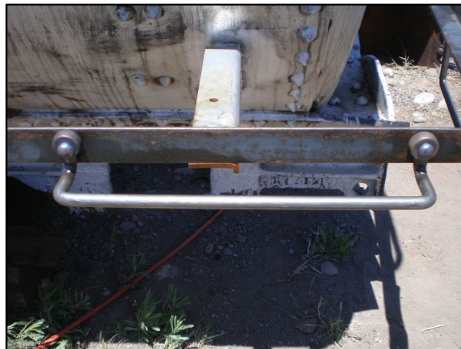
New grab iron riveted in place – just like the old days!
