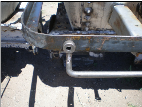
New grab iron in place – ready for a rivet.
