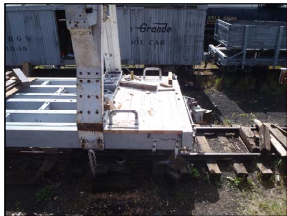
Outer supports/hold-downs have been reinstalled and secured – one on each side.
