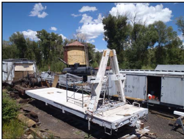
Car with the deck nailed down at the end of Session E.
