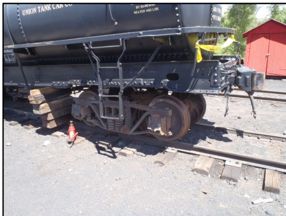
Arch-bar trucks have been moved under the tank car.
