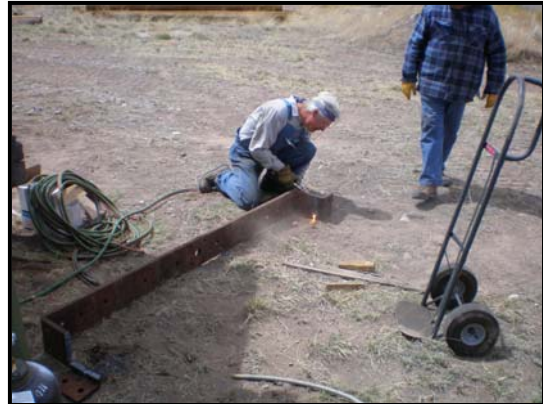
Mike Homer cutting bolster from 5510 for future use on 5995.
