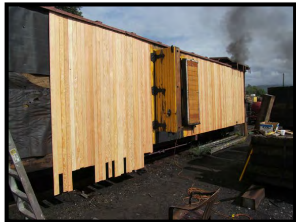
New paneling being installed.
