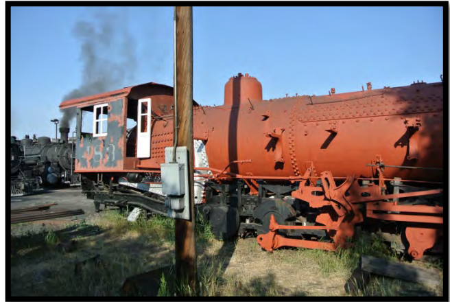
Engine 483 at the end of Session D shows a cab door and window installed.
