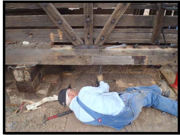
The splice in the side sill is perfect! You just can't get a better fit.
