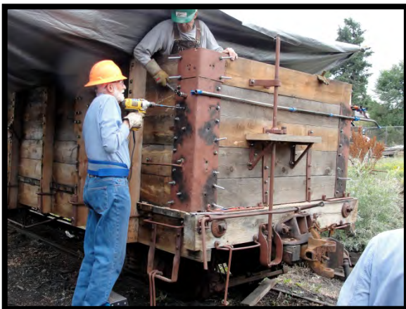
Warren Ringer drilling a hole for another bolt while John Sutkus tightens a nut.
