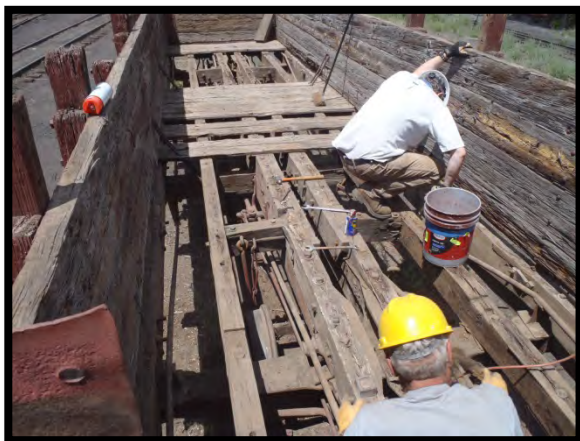
Rotten wood being removed from the floor.
