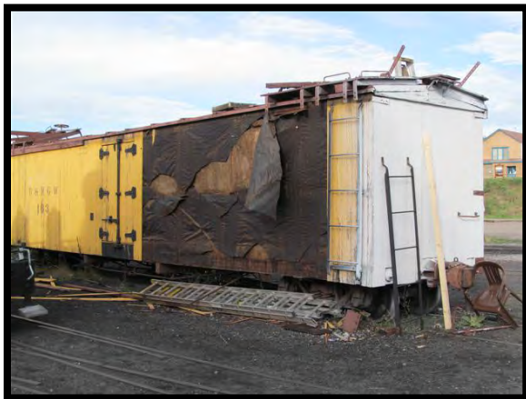
Old paneling being removed.
