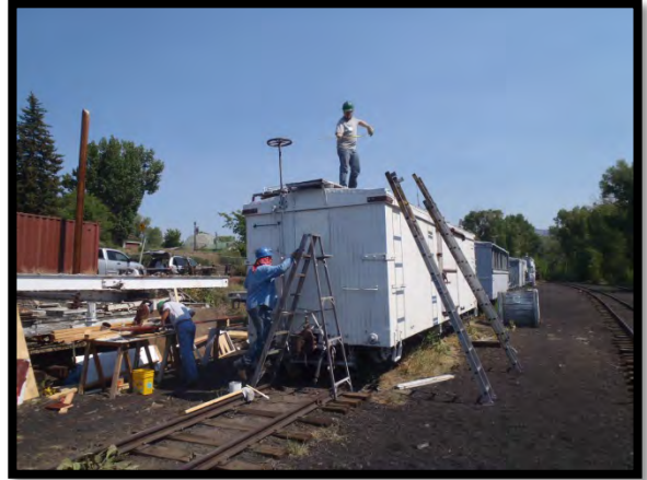
Bob Hayes is cutting a roof walk board. Dan Sandt, on the ladder, will be given another measurement for another roof walk board which was being taken by John Ferrell on top of the car.
