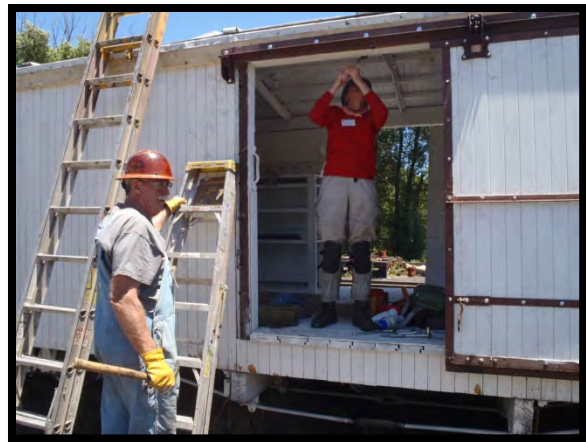
TL Craig McMullen has just finished tapping bolts through the car that holds the overhead door railing as Patricia Sandt tightens up the nuts on the inside of the car.
