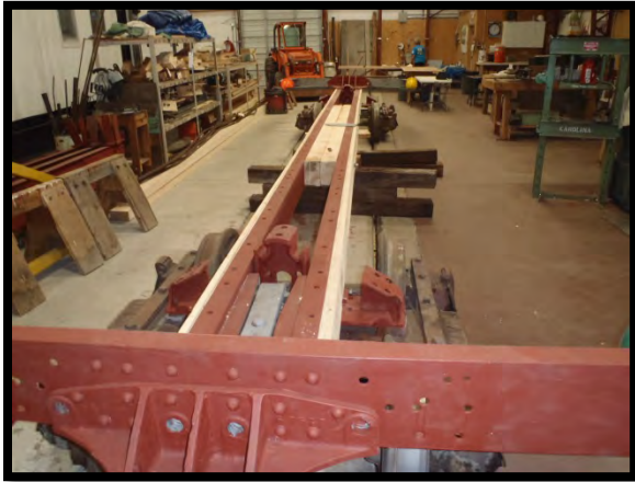
Center wood stiffing beams and two wood frame channel beams have been installed.
