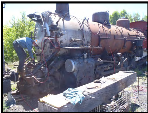
Mike McGinley using compressed air to blow various front end parts after rust, old paint, grime, etc. have been loosened.
