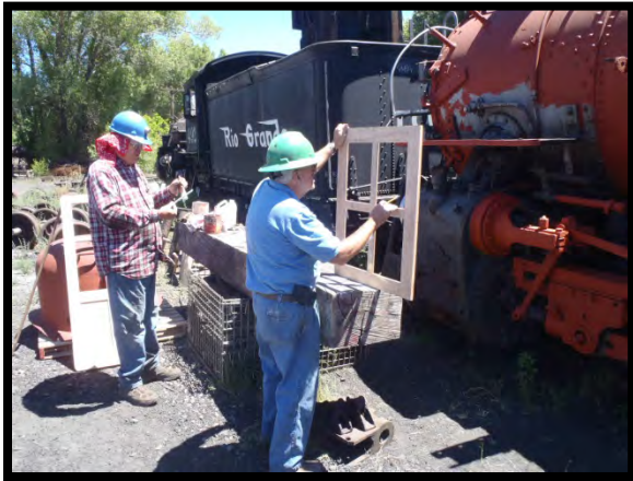
TL Dan Sandt and Bob Hayes work on a cab door and window built over the past winter by Jim Hickman.
