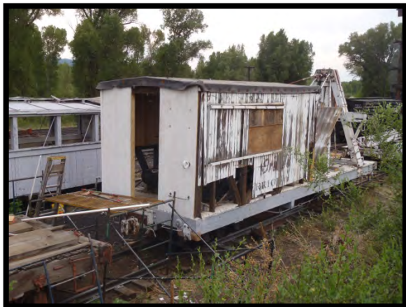
Siding has been installed on the B end.
