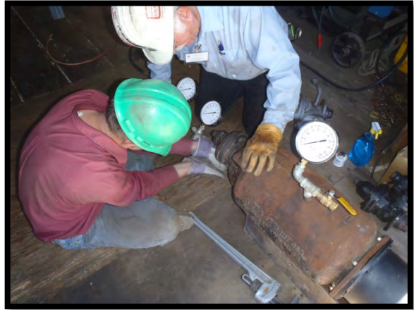
TL Clyde Putman and Chuck Duecker work on a newly built Triple Valve Test Stand.
