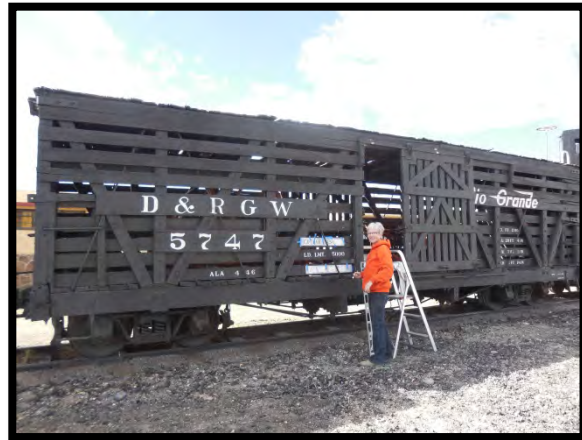
TL Valley Lowrance painting with stencil taped in the proper location on the car.
