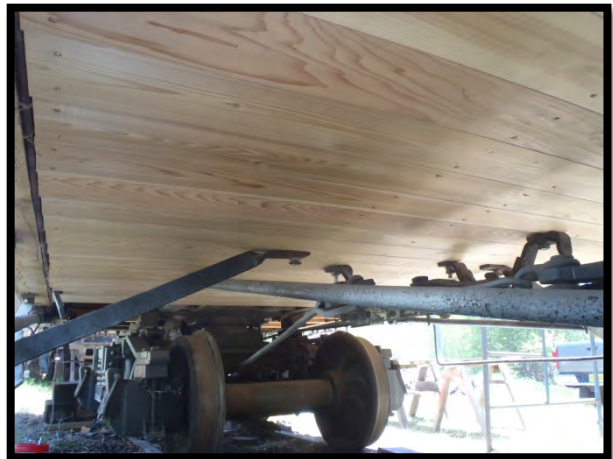
Fitting the wood underneath the car is no easy task – it's hard on old backs!
