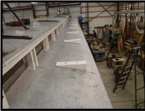
Roof walk blocks have been installed.
