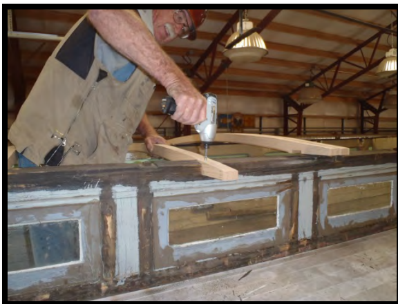
TL Craig McMullen screws down a carline using 3" #16 screws. New carlines were installed the full length of the roof.
