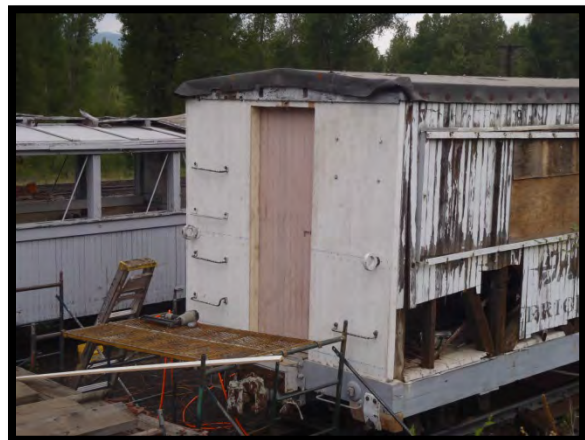
B end with the door installed – end of Session D
