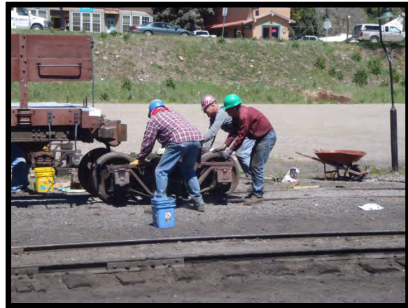
A better wheel set being moved under the car.
