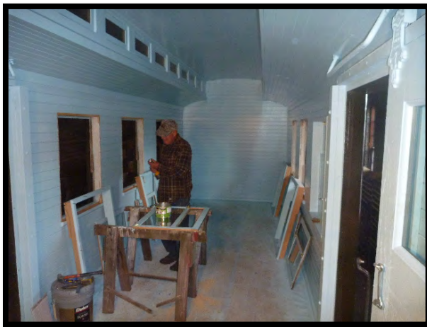
TL Don Bayer installing painted window frames.
