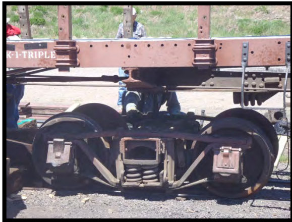
Cinder Bear Rider Gon #6205 an end has been raised in order to remove the wheel set.
