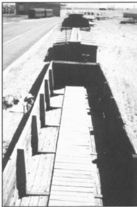
New flooring and side stakes were installed in the display train gondola at Antonito. July 1993. Photograph by Art Nichols.
