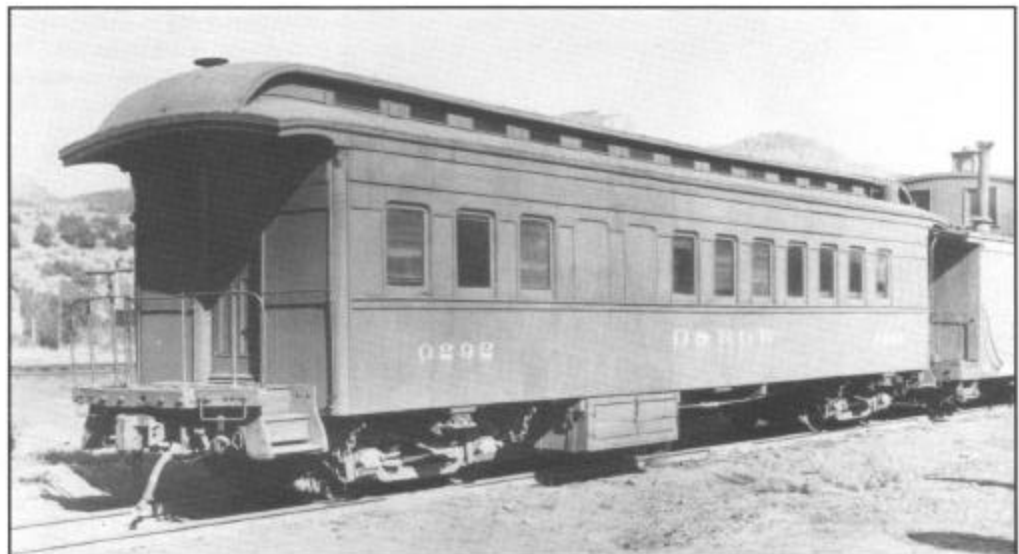
Passenger coach no. 0292 converted to maintenance-of-way, outfit service with the D&RGW. Note underbody storage bin. Gerald M. Best Collection, California State Railroad Museum.
