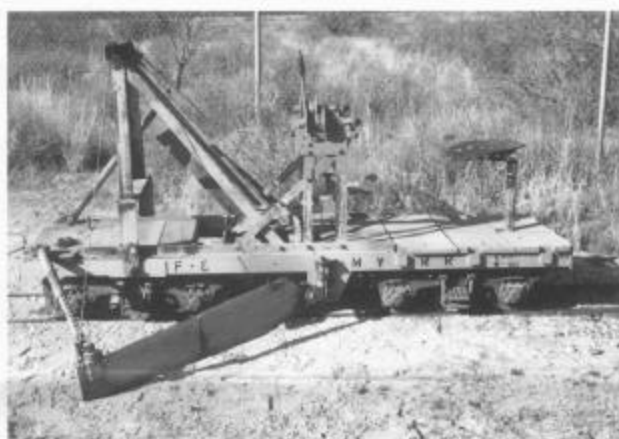
Jordan spreader, a must for preventing washouts.
