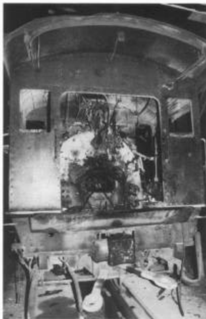
Engine 488 with backhead lagging removed, January 12, 1998.
