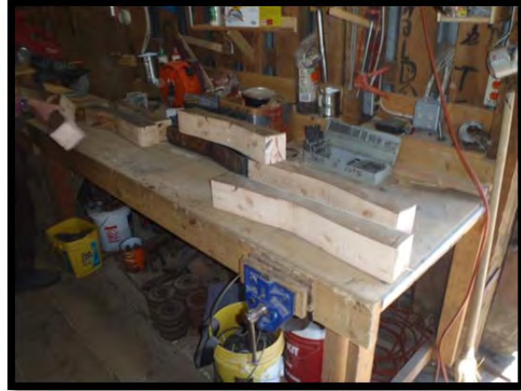
New roof walk cradles cut out and ready for drilling and painting before installation on sheep stock car #5633.
