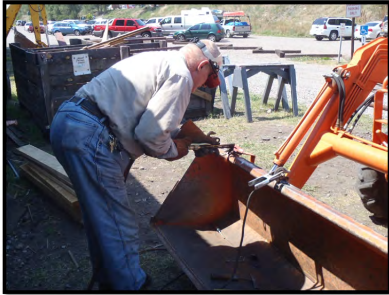
More torch work on the Kubota bucket.
