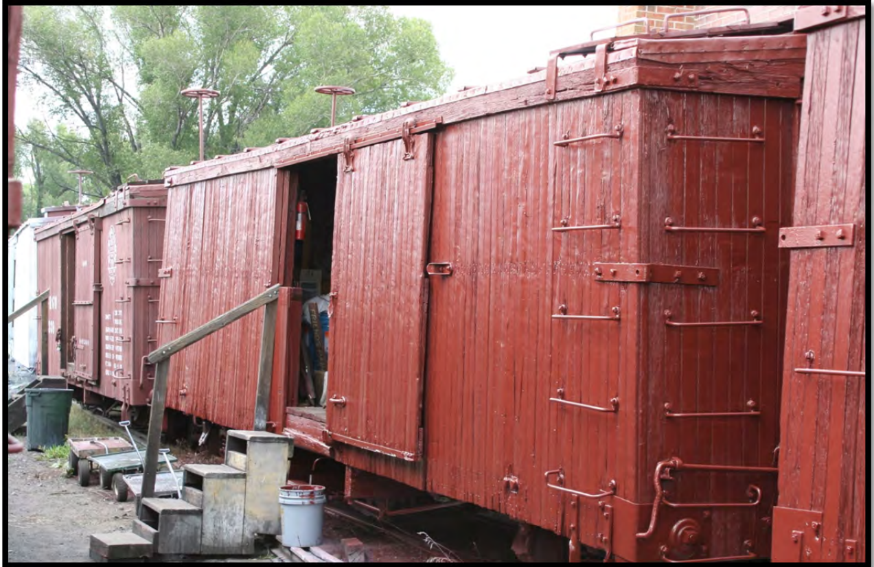
Boxcar 3669 (Project 1122) sides and ends were painted with a finish coat of Boxcar Red (Babbitt Brown). The primer and some finish color were applied to the car as it was being re-sided.
