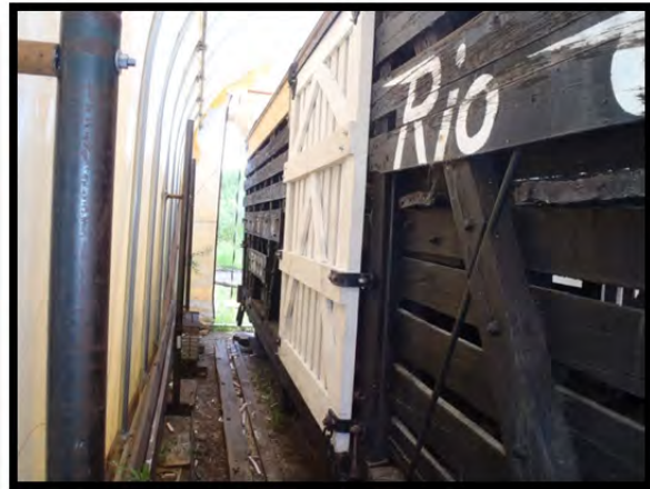
New door built by TL Jim Hickman primed in white. New doors were built for both sides and will be painted black during a later work session.
